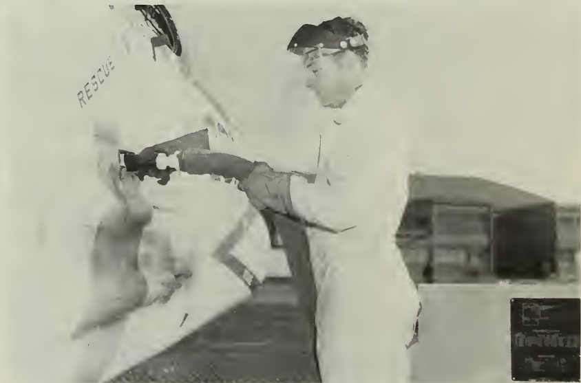
MACHINERY is set to blow off moisture separated from high pressure air during drying stage of production process. Rt: LOX is fed into jet's reservoir. When pilot needs oxygen LOX will be converted to gas, warmed for breathing.
